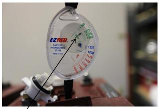
Use a hydrometer to get an accurate indication of how much charge is in the battery
