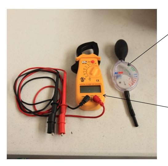
The hydrometer measures the gravity of the liquid in the battery. Easy to use and gives an accurate charge indication.
