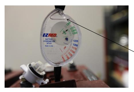
This is the proper level. Remember to shake the hydrometer a little to get any air bubbles out.
